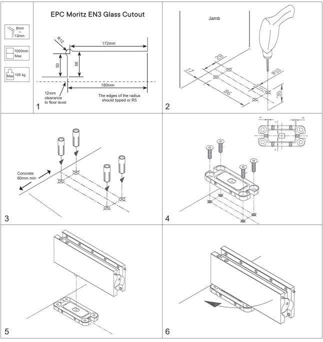
Once the patch is at 90° to the base the gaskets can be added and the door slid onto the patch and clamped in place by tightening up the screws on the
