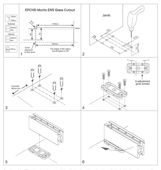
Once the patch is at  $90^{\circ}$  to the base the gaskets can be added and the door slid onto the patch and clamped in place by tightening up the screws on the
